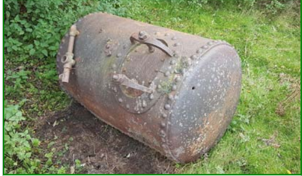
Air receiver on the surface at Penarth. (David Heavey)
