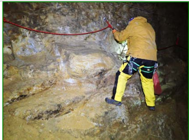
Stress testing a bolt using a 'standard' Holding (in his shiny new AV over trousers). (Vicky Robinson)
