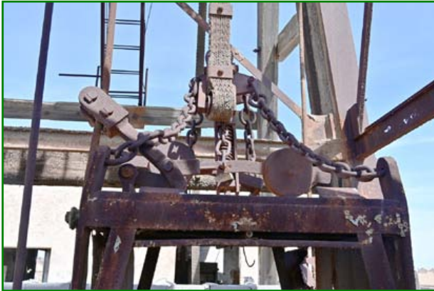
The cage suspension system at Pozo Carmelo.
