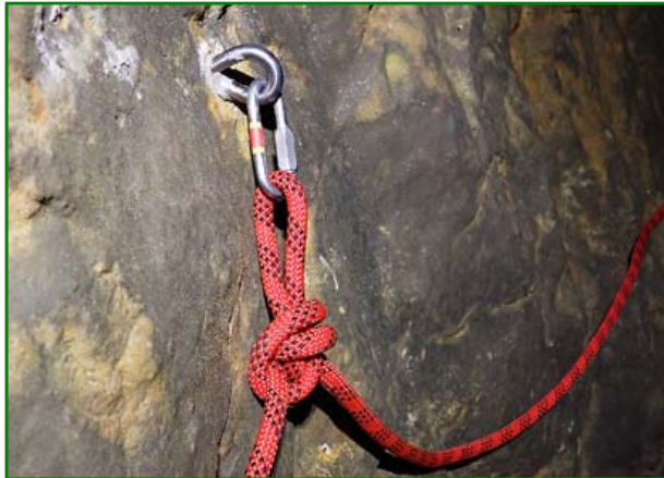
A finished bolt with maillon and rope. (Vicky Robinson)
