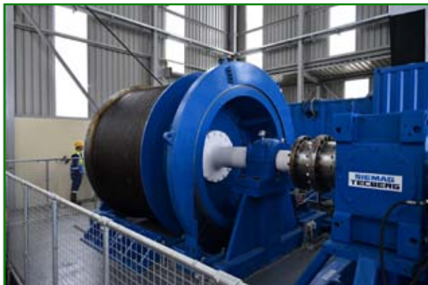
The current winding drum of the Roskear winding engine, NCK shaft. (Kelvin Lake)
