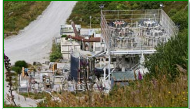
Hydro-cyclone refineries, Littlejohns mine. (Kelvin Lake)
