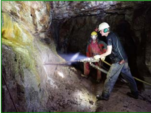
Demonstration of a Holman rock drill. (Vicky Robinson)
