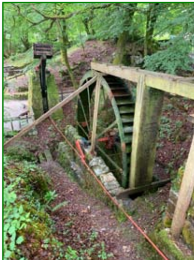
Waterwheel and iron 'flat' rod at Wheal Martyn. (Gareth Rushton)
