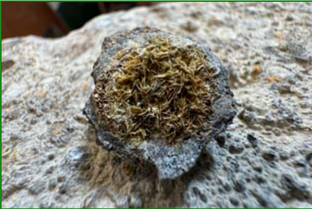
A 'blister' on a shipwreck tin ingot (~1cm diameter).
