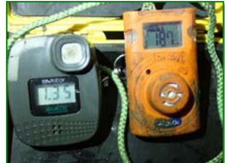
Carbon dioxide and oxygen readings near the 'County Gate'. (Steve Holding)
