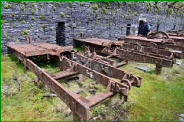
The saw tables - the belt drives came through wall slots.
