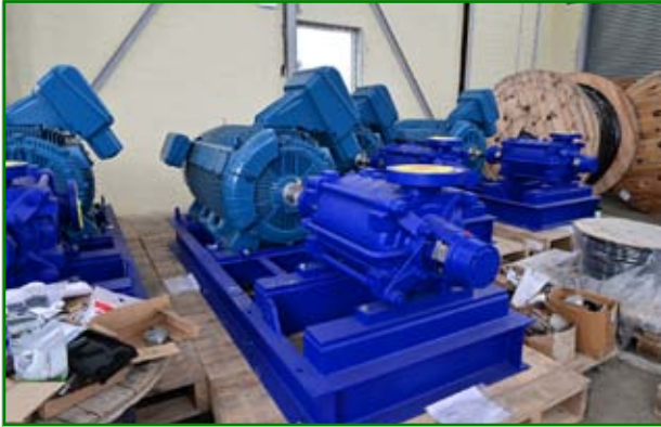
The new, larger pumps due to be installed at the 195 fathom level when water levels are low enough.
