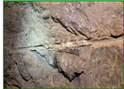
Shot hole with stemming still in place, Danby Level. (Vicky Robinson)
