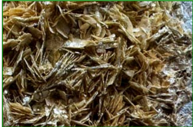
Detail of the Abhurite crystals in the blister.
