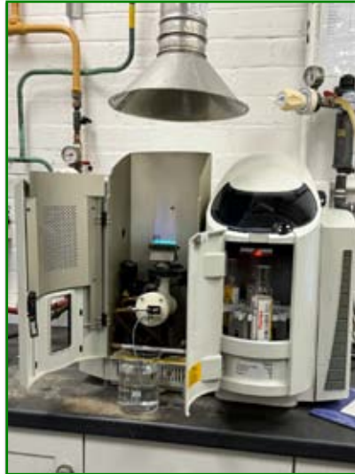
An Atomic Absorption Spectrometer in the Wheal Jane Lab.
