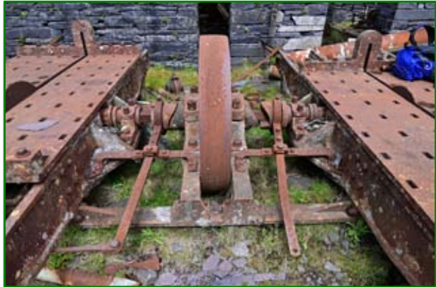
Saw table clutch mechanism and belt drive pulley.
