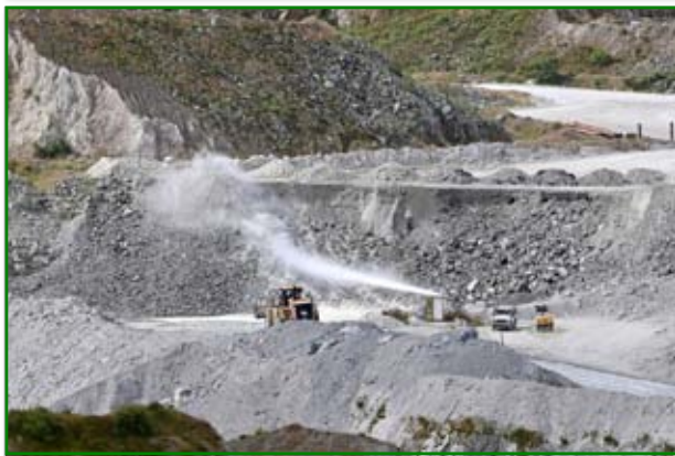
Hydraulic monitor at work in Littlejohns Kaolin Mine.
