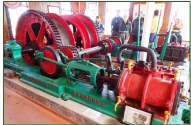
The Holman Bros. steam winder, now demonstrated with compressed air. (Vicky Robinson)
