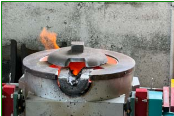
The tin is smelted in small gas furnace. (Kelvin Lake)
