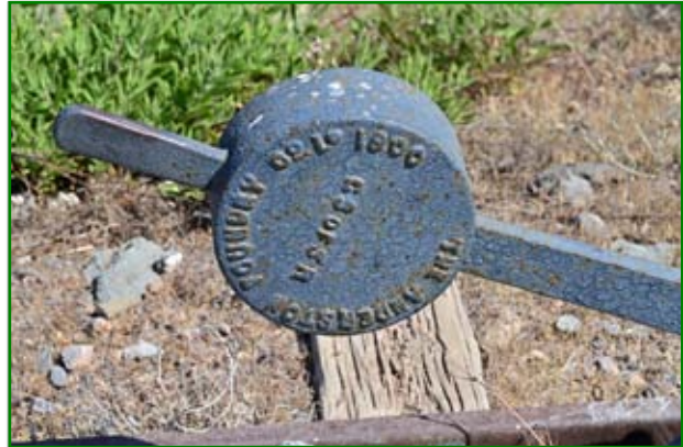
GSSR points lever by Alderston Foundry Co. Ltd., Glasgow & Middlesbro', 1899 (weight 1900).
