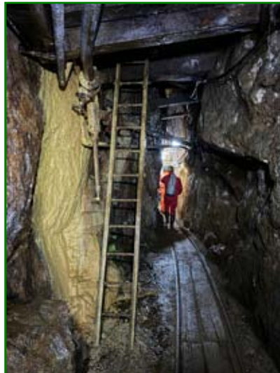
View along a tramming level below false floors in a stope. (Kelvin Lake)
