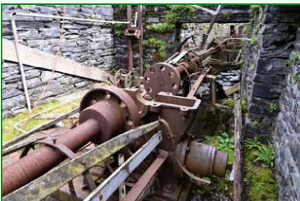
Lineshafting that drove the Australia mill saw tables.
