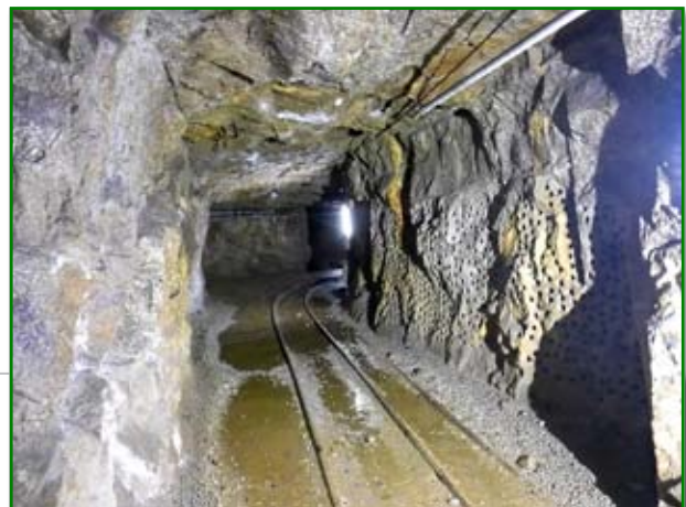
Typical access tunnel in Holman's Test mine with a large number of drill holes in the wall. (Julian Bromhead)
