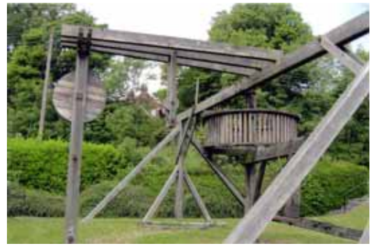
Figure 3, below: Horsegin at Bersham Museum, showing wheel, rolley pulley and drum with a 'lip' (Ivor Brown Collection)
