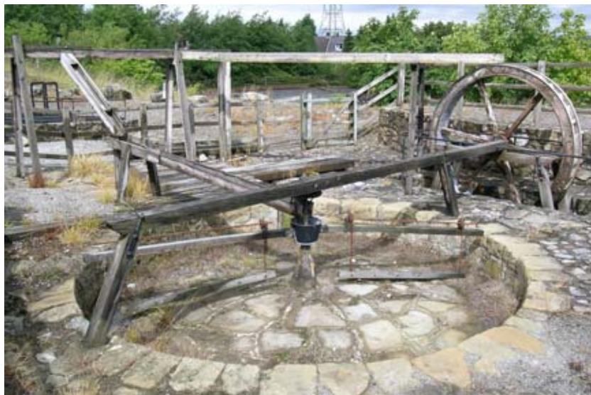
Below: A circular buddle at Minera Lead mine - the visitor centre here has one of Malcom Newtons models on loan from the Club, although it does not appear to be working any more.
