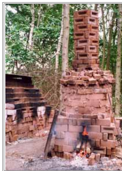
Above: Two experimental brick 'clamps' being fired at Maws Tileworks, May 2001, by A.J.Mugridge.
