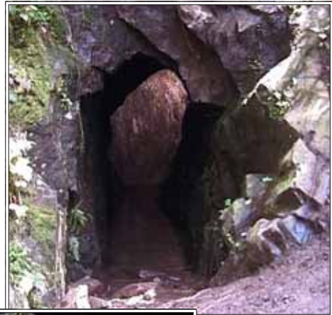
Right: View into La Torche Stolle - driven using firesetting. Note the irregular alignment of the level.
