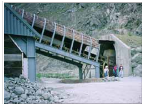
Left and Below: Main processing plant, conveyors and storage hoppers with loading bays for the graded rock.
