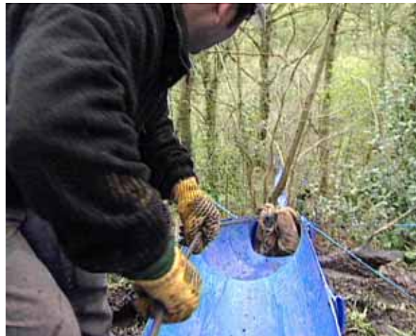
Above & left: Finished stone being sent down the logging chutes, wrapped in hessian sacking to protect it.
