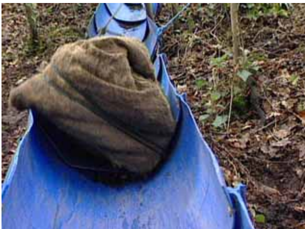
Above & left: Finished stone being sent down the logging chutes, wrapped in hessian sacking to protect it.
