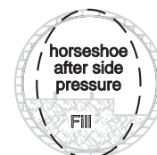
The Tar Tunnel as built (based on Gilpin 1796) and after side pressure (based on Brown 1974)
